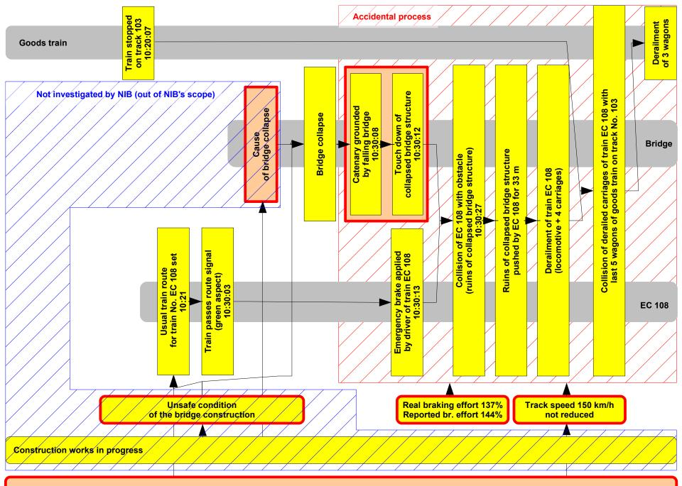
Risks originating from interaction between railway and construction site not mitigated (procedure not defined)
